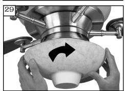
Attach glass by locating dimples in light kit with the groves in glass and twisting clockwise till tight.
